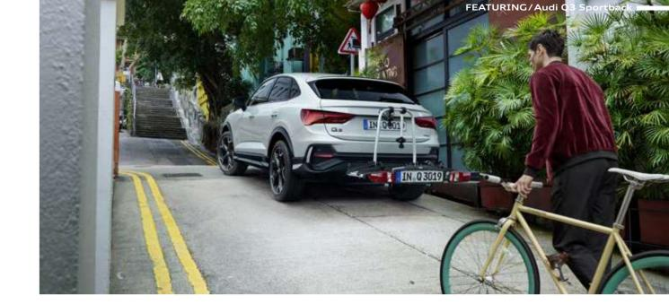
Transport bicycles and e-bikes easily and safely with the cycle rack for the trailer towing hitch: foldable and lockable; for 2 bicycles; extension set for a third bicycle available. Maximum load 60 kg.
